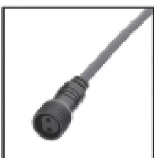
IP67 Connector 2PIN Wire Gauge : 0.326mm 2 /22AWG Protection : IP67 (Mated) Connector type : Female
